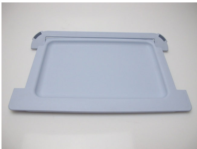
Photo 1: Lid for 6 L bucket (top view) after 40 autoclaving cycles
