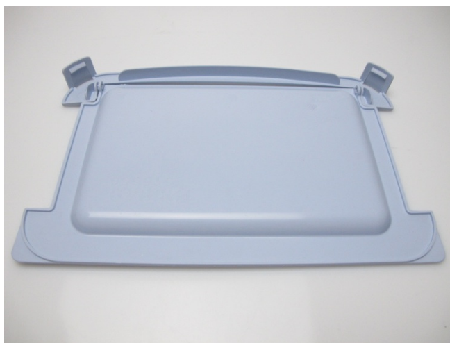
Photo 2: Lid for 6 L bucket (bottom view) after 40 autoclaving cycles
